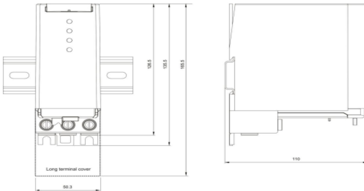
Figure 1: (Above) Dimensions of the E460 1ph DIN Rail G3-PLC meter
